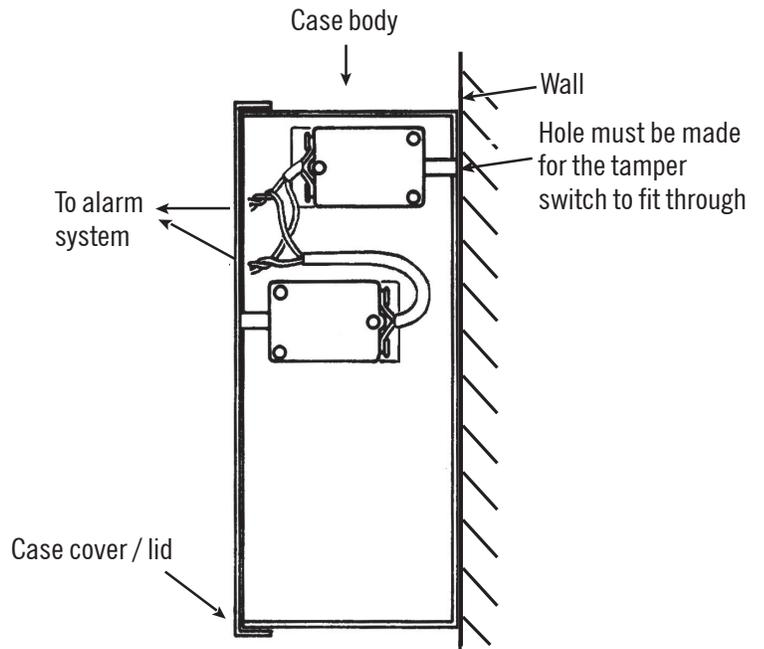
*Fig.3- Used inside box when top is opened upward or lifted off.*
